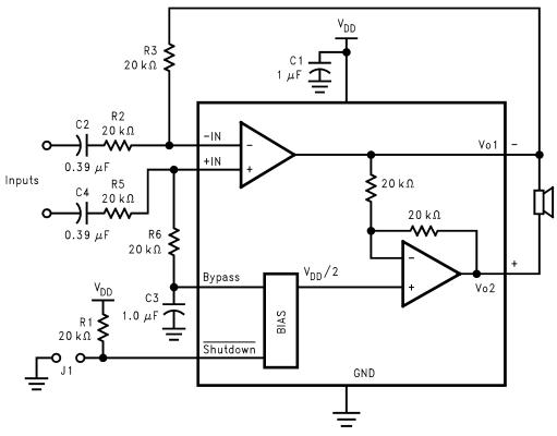
Figure 31. Differential Amplifier Configuration for LM4889
