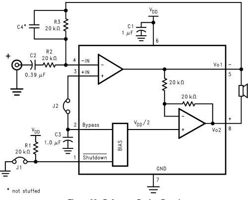
Figure 33. Reference Design Board
