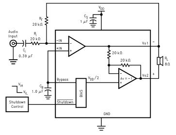
Figure 1. Typical Audio Amplifier Application Circuit
