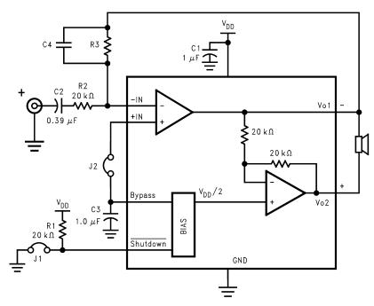
Figure 30. Higher Gain Audio Amplifier
