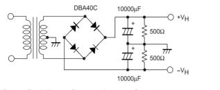
**Specified Transformer Power Supply** (MG-250 equivalent)
