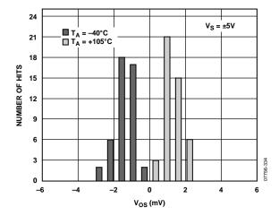
Figure 34. Input Offset Voltage Histogram over Temperature  $(V_5 = \pm 5 V)$ , SOIC Only
