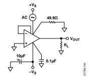
Figure 47. Positive Power Supply Rejection
