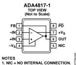
Figure 2. 8-Lead SOIC (RD-8-1)
