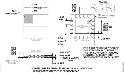
Figure 73.16-Lead Lead Frame Chip Scale Package [LFCSP] 4 mm × 4 mm Body and 0.75 mm Package Height (CP-16-20) Dimensions shown in millimeters
