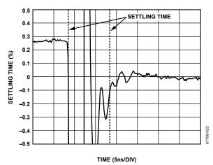
Figure 24. 0.1% Short-Term Settling Time
