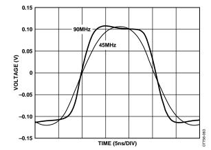
Figure 69. Small Signal Transient Response (Low-Pass Filter)
