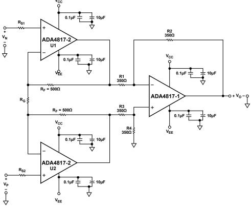
Figure 66. High Speed Instrumentation Amplifier
