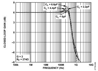
Figure 10. Small Signal Frequency Response for Various C<sub>L</sub>
