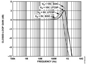
Figure 9. Small Signal Frequency Response for Various Supplies
