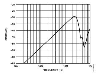
Figure 26. Common-Mode Rejection Ratio (CMRR) vs. Frequency
