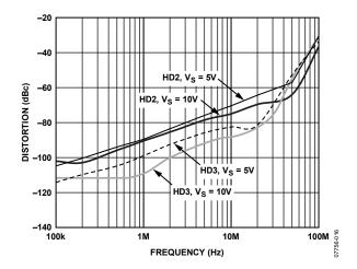
Figure 16. Distortion vs. Frequency for Various Supplies, G = 2,  $V_{OUT} = 2 V p-p$
