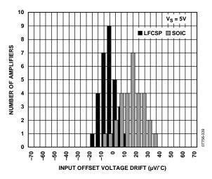
Figure 42. Input Offset Voltage Drift Histogram  $(V_S = 5 V)$
