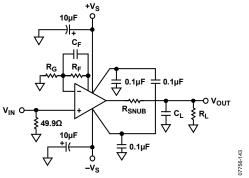
Figure 56. R<sub>SNUB</sub> or C<sub>F</sub> Used to Reduce Peaking
