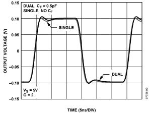
Figure 22. Small Signal Transient Response
