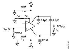
Figure 49. Noninverting Gain Configuration
