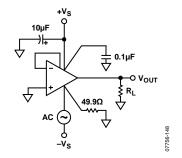
Figure 50. Negative Power Supply Rejection
