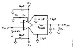
Figure 48. Capacitive Load Configuration
