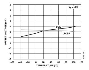
Figure 38. Offset Voltage vs. Temperature  $(V_S = \pm 5 V)$
