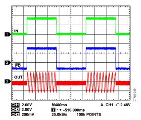
Figure 58. Power-Down Operation
