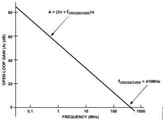
Figure 54. Open-Loop Gain vs. Frequency
