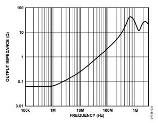
Figure 27. Output Impedance vs. Frequency
