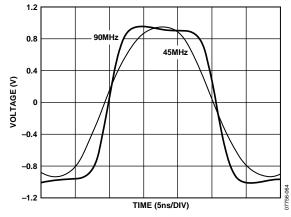
Figure 70. Large Signal Transient Response (Low-Pass Filter)
