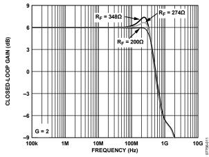
Figure 13. Small Signal Frequency Response for Various R<sub>F</sub>
