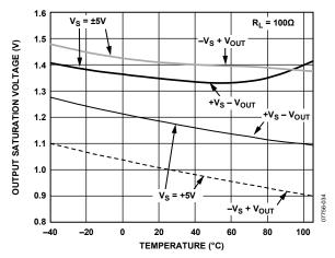
Figure 30. Output Saturation Voltage vs. Temperature
