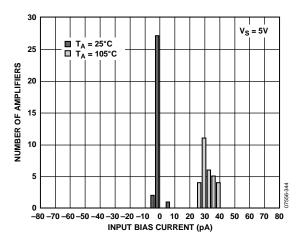
Figure 43. Input Bias Current Histogram over Temperature (VS = 5 V)
