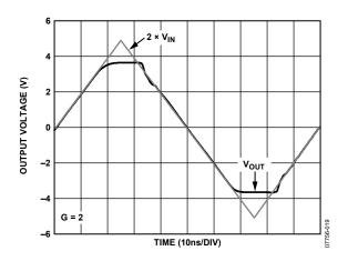
Figure 21. Output Overdrive Recovery
