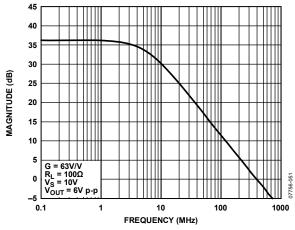
Figure 65. Photodiode Preamp Frequency Response
