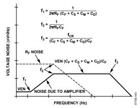
Figure 64. Photodiode Voltage Noise Contributions
