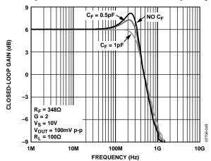
Figure 59. Small Signal Frequency Response vs. Feedback Capacitor
