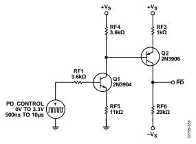
Figure 57. Power-Down Circuit
