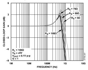
Figure 60. Small Signal Frequency Response for Various R<sub>5</sub> (SOIC)
