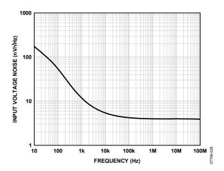
Figure 28. Input Voltage Noise vs. Frequency
