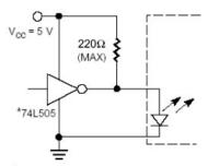
\*ANY OPEN COLLECTOR TTL OR OPEN DRAIN CMOS GATE.
