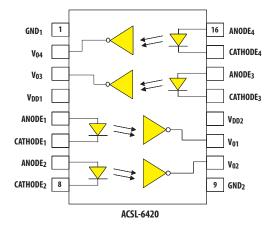
A 0.1- $\mu$ F bypass capacitor must be connected as close as possible between the power supply pins, VDD and GND, VDD1 and GND1, VDD2 and GND2.
