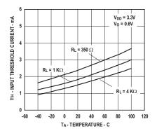
Figure 18: Typical Input threshold Current vs. Temperature for 5V Operation
