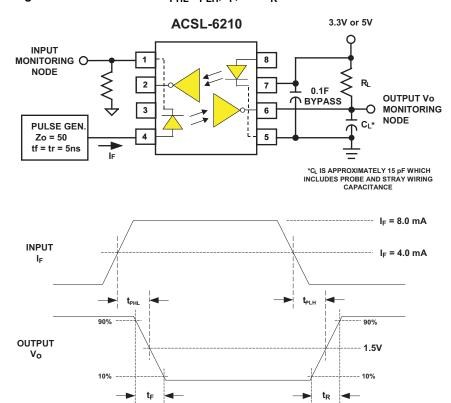
Figure 33: Test Circuit for Common Mode Transient Immunity and Typical Waveforms
