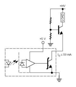
Figure 38: High Voltage and High Current Switching with ACSL-6xx0
