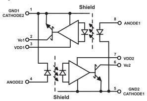
secondary amplifier stage of the detector IC feeds into an open collector Schottky-clamped transistor.
