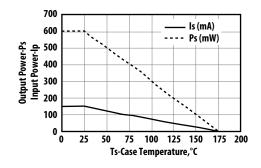
This optocoupler is suitable for safe electrical isolation only within the safety limit data. Maintenance of the safety data shall be ensured by means of protective circuits.
