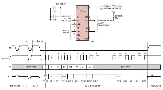
Figure 7. Internal Serial Clock, Single Cycle Operation
