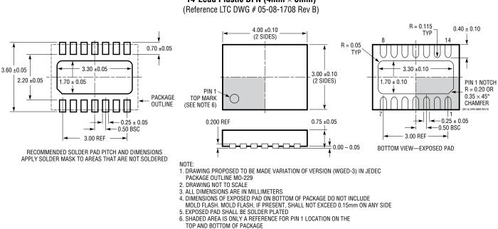
DE Package 14-Lead Plastic DFN (4mm × 3mm) Reference LTC DWG # 05-08-1708 Rev P)
