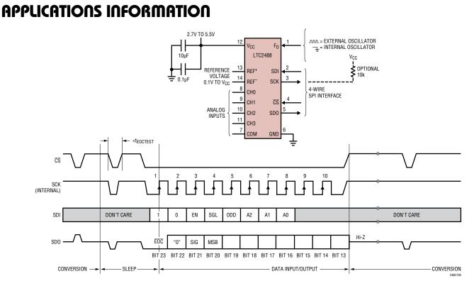
Figure 8. Internal Serial Clock, Reduced Data Output Length with Valid Channel and Configuration Selection
