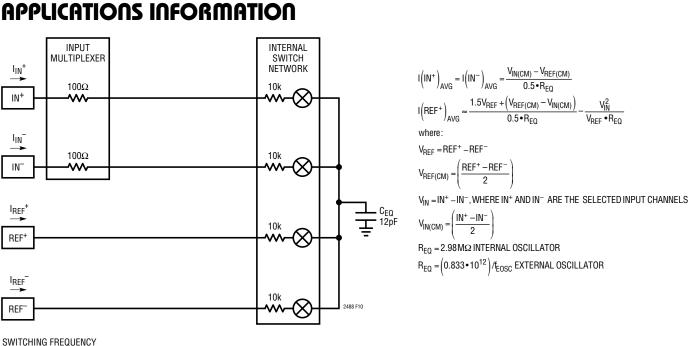
f<sub>SW</sub> = 123kHz INTERNAL OSCILLATOR
