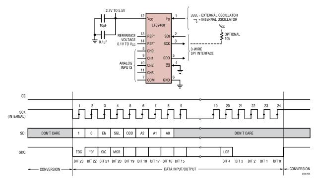
Figure 9. Internal Serial Clock, Continuous Operation
