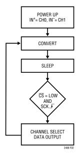
Figure 2. LTC2488 State Transition Diagram
