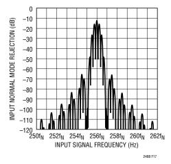
Figure 17. Input Normal Mode Rejection at  $f_S = 256 \bullet f_N$
