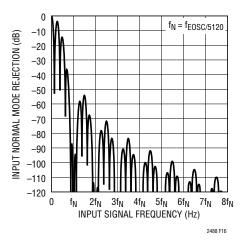
Figure 16. Input Normal Mode Rejection at DC
