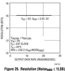
vs Output Data Rate and Reference Voltage
