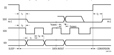
Timing Diagram Using Internal SCK (SCK HIGH with  $\overline{\text{CS}}\downarrow$ )
