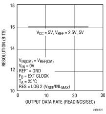
Figure 27. Resolution (INL<sub>MAX</sub>  $\leq$  1LSB) vs Output Data Rate and Reference Voltage
