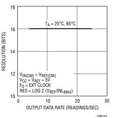
Figure 24. Resolution (INL<sub>MAX</sub>  $\leq$  1LSB) vs Output Data Rate and Temperature
