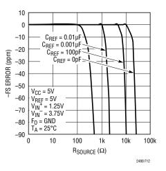
Figure 12. –FS Error vs  $R_{SOURCE}$  at  $V_{REF}$  (Small  $C_{REF}$ )
