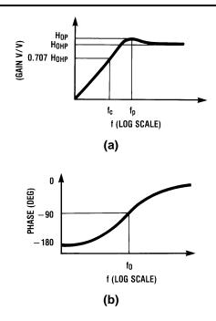
$$\begin{split} & \textbf{H}_{HP}(\textbf{s}) = \frac{\textbf{H}_{OHP}\textbf{s}^2}{\textbf{s}^2 + \frac{\textbf{s}\omega_O}{Q} + \omega_O{}^2} \\ & \textbf{f}_C = \textbf{f}_O \times \left[ \sqrt{\left(1 - \frac{1}{2Q^2}\right) + \sqrt{\left(1 - \frac{1}{2Q^2}\right)^2 + 1}} \, \right]^{-1} \\ & \textbf{f}_p = \textbf{f}_O \times \left[ \sqrt{1 - \frac{1}{2Q^2}} \right]^{-1} \\ & \textbf{H}_{OP} = \textbf{H}_{OHP} \times \frac{1}{\frac{1}{Q}\sqrt{1 - \frac{1}{4Q^2}}} \end{split}$$
