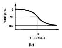
$$\begin{split} H_{LP}(s) &= \frac{H_{OLP}\omega_{O}^{2}}{s^{2} + \frac{s\omega_{O}}{Q} + \omega_{O}^{2}} \\ f_{C} &= f_{O} \times \sqrt{\left(1 - \frac{1}{2Q^{2}}\right) + \sqrt{\left(1 - \frac{1}{2Q^{2}}\right)^{2} + 1}} \\ f_{p} &= f_{O} \sqrt{1 - \frac{1}{2Q^{2}}} \\ H_{OP} &= H_{OLP} \times \frac{1}{\frac{1}{Q}\sqrt{1 - \frac{1}{4Q^{2}}}} \end{split}$$
