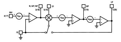
Figure 35. MF10-N Offset Voltage Sources
