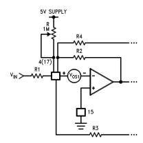
Figure 36. Method for Trimming Vos
