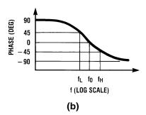
$$\begin{split} & \textbf{H}_{BP}(\textbf{s}) = \frac{\textbf{H}_{OBP} \frac{\omega O}{Q} \, \textbf{S}}{\textbf{s}^2 + \frac{\textbf{s}\omega_O}{Q} + \, \omega_O^2} \\ & \textbf{Q} = \frac{f_O}{f_H - f_L}; \,\, f_O = \sqrt{f_L f_H} \\ & \textbf{f}_L = f_O \left( \frac{-1}{2Q} + \sqrt{\left(\frac{1}{2Q}\right)^2 + 1} \,\, \right) \\ & \textbf{f}_H = f_O \left( \frac{1}{2Q} + \sqrt{\left(\frac{1}{2Q}\right)^2 + 1} \,\, \right) \\ & \omega_O = 2\pi f_O \end{split}$$
