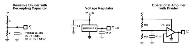
Figure 34. Three Ways of Generating V<sup>+</sup>/2 for Single-Supply Operation
