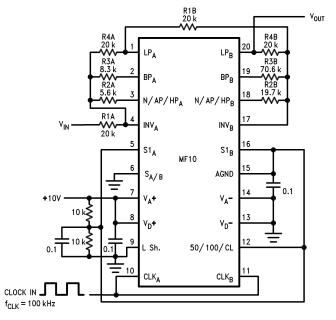
Figure 33. Fourth-Order Chebyshev Low-Pass Filter from Example in 3.1.
