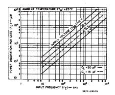
Fig.2 - Typical power dissipation vs. frequency.
