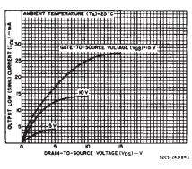
Fig.3 – Typical output low (sink) current characteristics.
