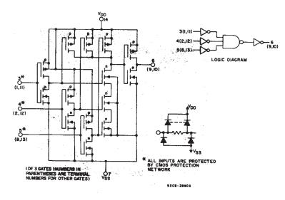
Fig. 7 - Schematic and logic diagrams for CD4025B.
