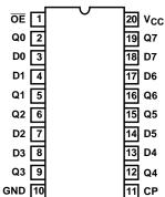
CD54HC574, CD54HCT574 (CERDIP) CD74HC574 (PDIP, SOIC) CD74HCT574 (PDIP, SOIC, TSSOP) TOP VIEW
