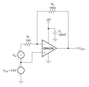
Figure 25. Basic Single-Supply Connection
