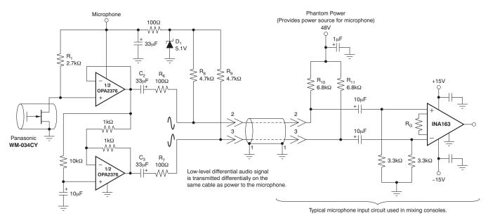
Figure 28. Phantom-Powered Electret Microphone
