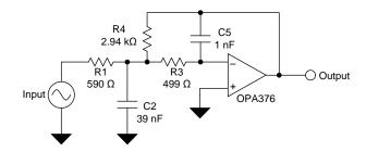
Figure 30. Typical Application Schematic
