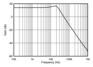
Figure 31. Low-Pass Filter Transfer Function
