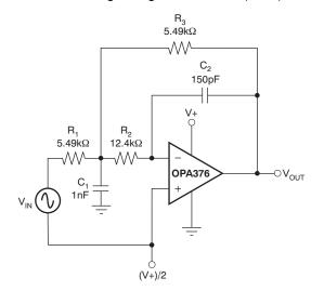
Figure 26. Second-Order, Butterworth, 50-kHz, Low-Pass Filter
