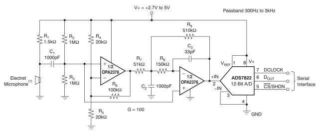
(1) Electret microphone powered by R<sub>1</sub>.
