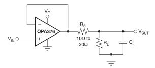
Figure 22. Improving Capacitive Load Drive
