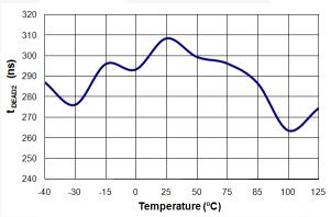
Figure 40. t<sub>DEAD1</sub> (R<sub>RP</sub>=43 k, 2.5 μs) vs. T<sub>A</sub>
