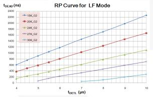
Figure 5. t<sub>DEAD</sub> vs. t<sub>DETL</sub> RP Curve for LF Mode
