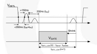
Figure 15. Gate Shrink by DETL Voltage Ringing Around Zero
