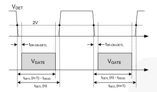
Figure 10.SR Gate Timing Diagram
