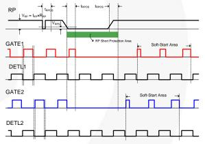
Figure 17. RP Pin Short Protection
