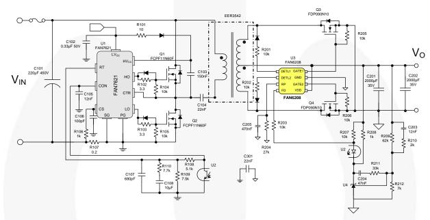
Figure 44. Application Circuit
