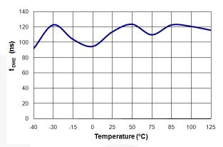
Figure 32.  $t_{\text{DW1}}$  vs.  $T_{\text{A}}$
