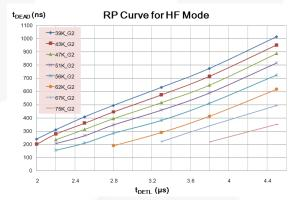
Figure 6. t<sub>DEAD</sub> vs. t<sub>DETL</sub> RP Curve for HF Mode
