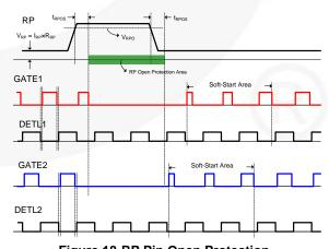
Figure 18.RP Pin Open Protection
