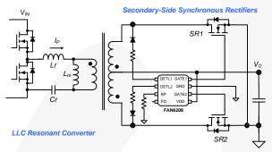
Figure 7. Simplified Schematic of LLC Converter
