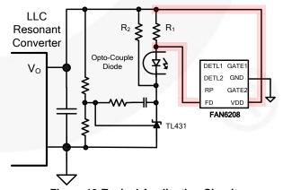
Figure 13. Typical Application Circuit
