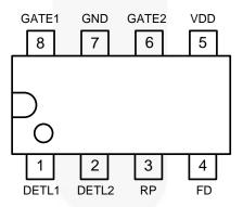
Figure 4. Pin Assignments
