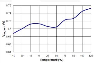
Figure 22. V<sub>TH OFF1</sub> vs. T<sub>A</sub>
