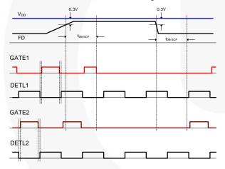
Figure 19. Output Short Protection by Feedback Detection
