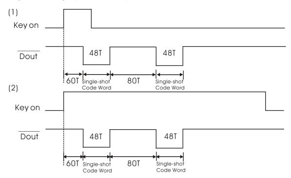
When any one of the single-shot key is pressed, it will transmit the command word in 2 cycles, and end the transmitting.
