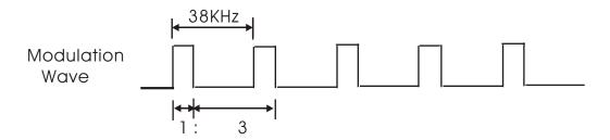
Fcarrier wave = fosc/12(fosc = 455KHz, fcarrier wave
