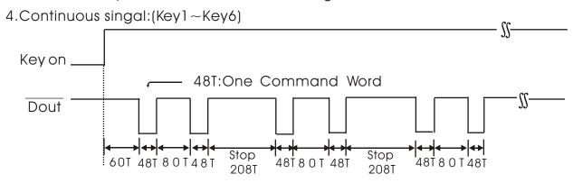
When any one of the continuous key is pressed, it will transmit the command word in 2 cycle, but it will repeat the output until the key is deprssed. (The latest 2 command code word must be output completely)
