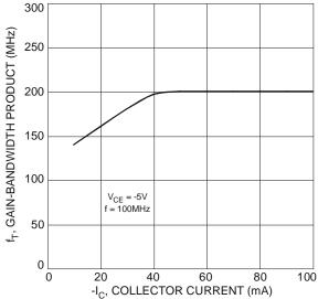
Fig. 6 Typical Gain-Bandwidth Product vs. Collector Current
