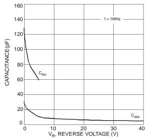
Fig. 7 Typical Capacitance Characteristics
