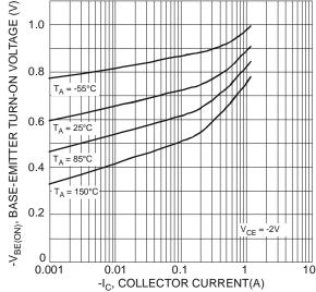
Fig 3 Typical Base-Emitter Turn-On Voltage vs. Collector Current
