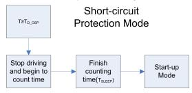
Figure 14 Flow Diagram of Short-circuit Protection Mode
