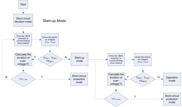
Figure 12 Flow Diagram of Start-up Mode
