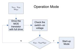
Figure 13 Flow Diagram of Operation Mode
