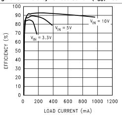
Figure 18. Efficiency vs Load ( $V_{OUT} = 15 V$ ) - "Y"
