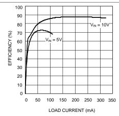
Figure 15. Efficiency vs Load Current (V<sub>OUT</sub> = 30 V) - "X"
