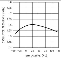
Figure 3. Oscillator Frequency vs Temperature - "X"
