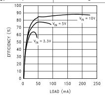
Figure 23. Efficiency vs Load (V<sub>OUT</sub> = 40 V) - "Y"
