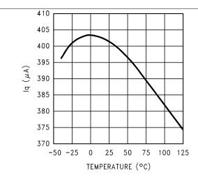
Figure 1. Iq  $V_{\text{IN}}$  (Active) vs Temperature - "X"
