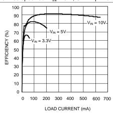
Figure 13. Efficiency vs Load Current (V<sub>OUT</sub> = 20 V) - "X"
