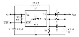
Figure 24. Basic Application Circuit
