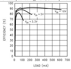
Figure 19. Efficiency vs Load (V<sub>OUT</sub> = 20 V) - "Y"
