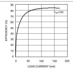
Figure 17. Efficiency vs Load Current (V<sub>OUT</sub> = 40 V) - "X"
