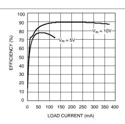
Figure 14. Efficiency vs Load Current (V<sub>OUT</sub> = 25 V) - "X"
