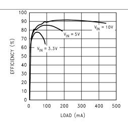
Figure 20. Efficiency vs Load (V<sub>OUT</sub> = 25 V) - "Y"
