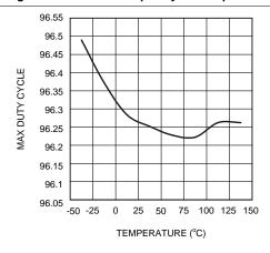
Figure 6. Max. Duty Cycle vs Temperature - "Y"
