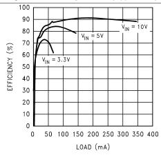
Figure 21. Efficiency vs Load (V<sub>OUT</sub> = 30 V) - "Y"
