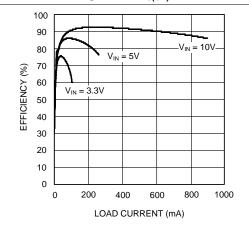
Figure 11. Efficiency vs Load Current (V<sub>OUT</sub> = 12 V) - "X"
