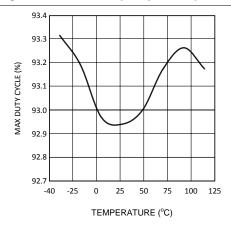
Figure 5. Max. Duty Cycle vs Temperature - "X"
