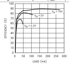
Figure 22. Efficiency vs Load (V<sub>OUT</sub> = 35 V) - "Y"
