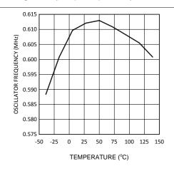
Figure 4. Oscillator Frequency vs Temperature - "Y"
