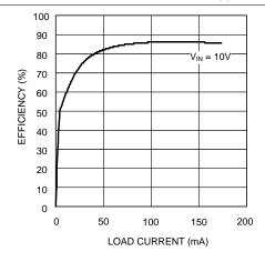
Figure 16. Efficiency vs Load Current (V<sub>OUT</sub> = 35 V) - "X"
