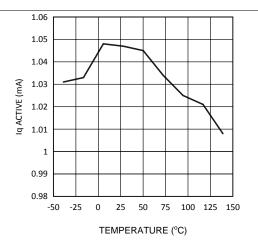
Figure 2. Iq V<sub>IN</sub> (Active) vs Temperature - "Y"
