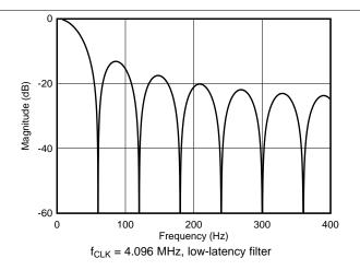
Figure 61. Low-Latency Filter Frequency Response,
