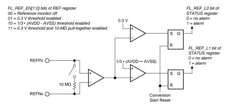
Figure 79. Reference Monitor Block Diagram
