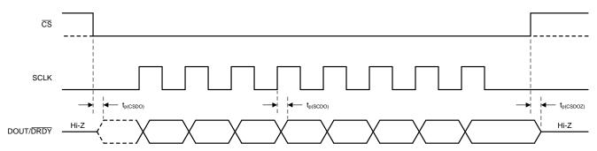
NOTE: Single-byte communication is shown. Actual communication can be multiple bytes.
