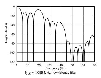
Figure 55. Low-Latency Filter Frequency Response, Data Rate = 5 SPS
