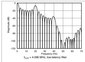
Figure 54. Low-Latency Filter Frequency Response, Data Rate = 2.5 SPS
