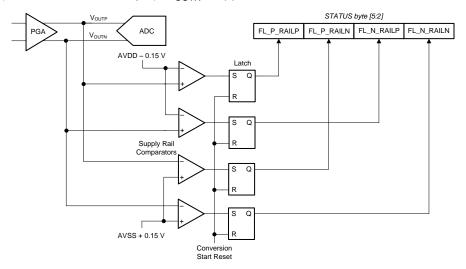
Figure 77. PGA Output Voltage Rail Monitors
