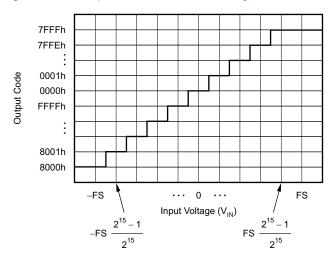
Figure 87. Code Transition Diagram
