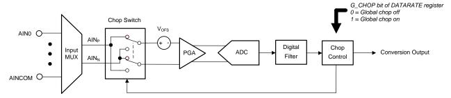
Figure 73. ADC Global Chop Block Diagram
