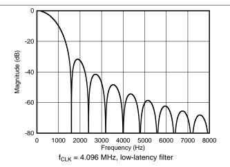
Figure 65. Low-Latency Filter Frequency Response,
