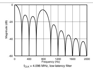
Figure 63. Low-Latency Filter Frequency Response,
