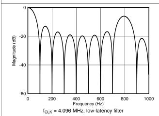
Figure 62. Low-Latency Filter Frequency Response, Data Rate = 100 SPS
