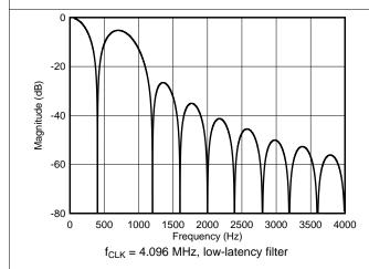
Figure 64. Low-Latency Filter Frequency Response,
