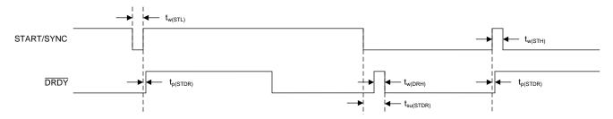
Figure 4. START/SYNC Pin Timing Requirements
