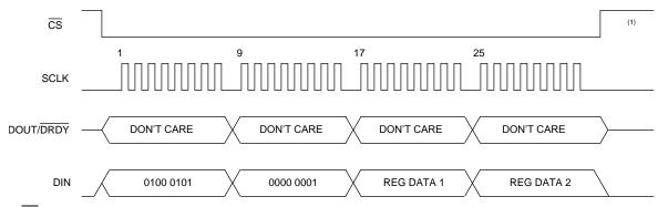
(1) CS can be set high or kept low between commands. If kept low, the command must be completed.
