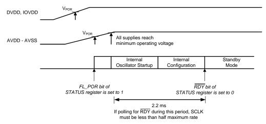
Figure 83. Power-On Reset Timing Sequence
