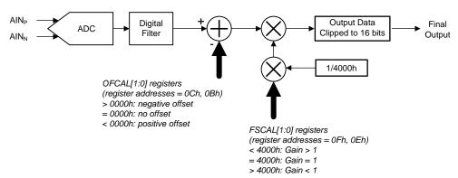
Figure 81. ADC Calibration Block Diagram
