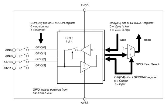
Figure 80. GPIO Block Diagram
