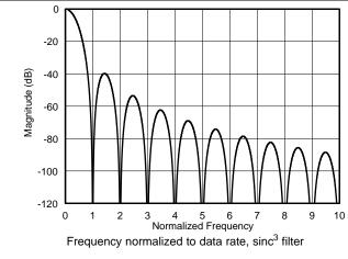
Figure 69. Sinc<sup>3</sup> Filter Frequency Response, Normalized to Data Rate
