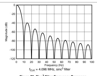
Figure 70. Sinc<sup>3</sup> Filter Frequency Response, Data Rate = 10 SPS
