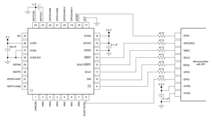
Figure 111. Serial Interface Connections
