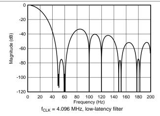
Figure 58. Low-Latency Filter Frequency Response,
