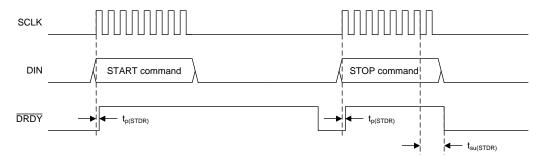
Figure 5. START Command Timing Requirements
