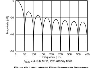
Figure 60. Low-Latency Filter Frequency Response,
