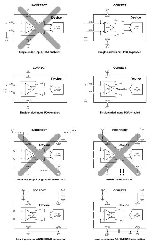
Figure 117. Do's and Don'ts Circuit Connections
