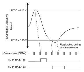
Figure 78. PGA Output Voltage Rail Monitor Timing
