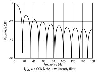
Figure 57. Low-Latency Filter Frequency Response,
