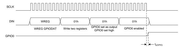
Figure 7. GPIO Switching Characteristics
