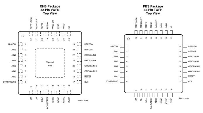
NOTE: The analog input functions (AIN6-AIN11) are not available on pins 19 to 22, 31, and 32 for the ADS114S06.
