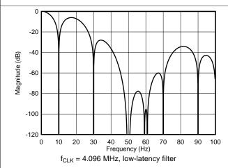
Figure 56. Low-Latency Filter Frequency Response, Data Rate = 10 SPS
