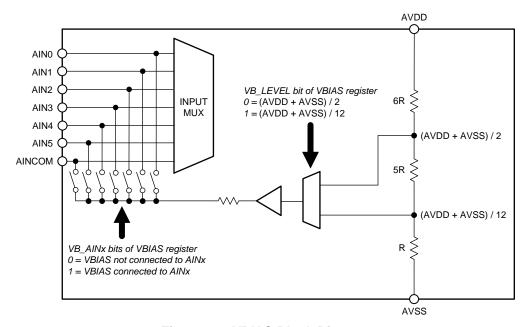
Figure 76. VBIAS Block Diagram
