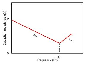
Figure 8-4. Capacitor Impedance versus Frequency
