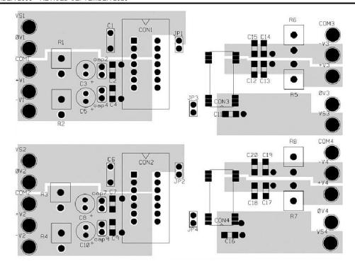
Figure 10-3. PCB Layout Example, Component-Side View
