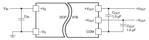
Figure 7-7. Dual Output Devices Connected in Series
