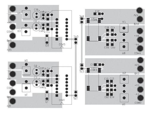
Figure 10-4. PCB Layout Example, Non-Component-Side View
