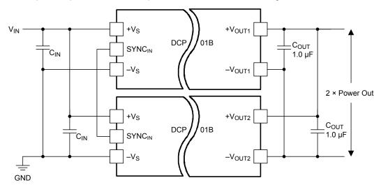
Figure 7-8. Multiple DCP01B Devices Connected in Parallel
