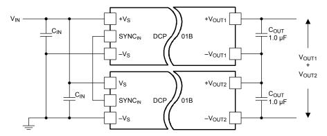
Figure 7-6. Multiple DCP01B Devices Connected in Series
