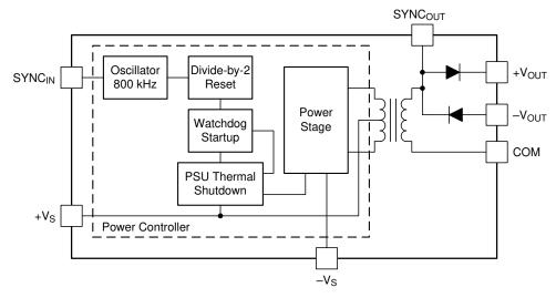
Figure 7-2. Dual Output Device
