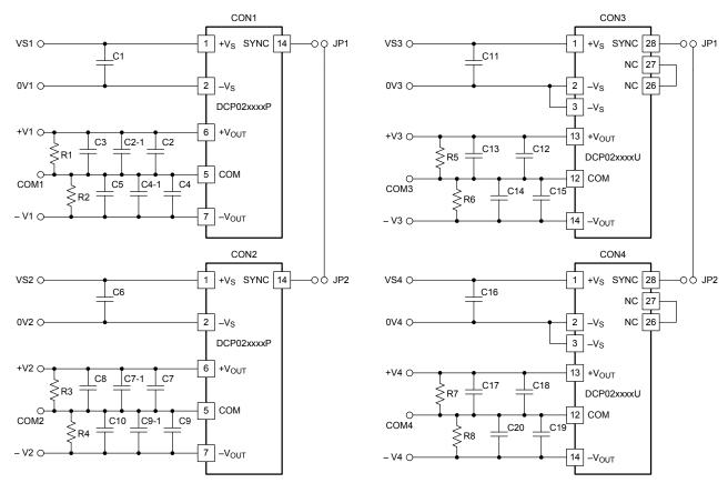
Figure 10-1. PCB Schematic, P Package
