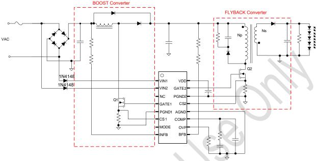
Fig.1 A typical isolated lighting application circuit
