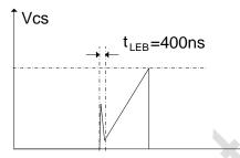
Fig.3 Leading-Edge Blanking
