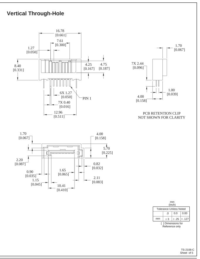
Signal Plug, Boardmount, Surface Mount Right Angle and PTH Vertical
