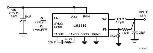
FIGURE 1. Typical Circuit for 1.8V Output Voltage
