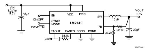
FIGURE 2. Typical Circuit for 2.5V Output Voltage
