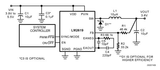
FIGURE 4. Typical Operating Circuit for 3.6V Output Voltage
