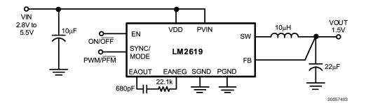
FIGURE 3. Typical Circuit for 1.5V Output Voltage
