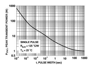
Figure 12. Single Pulse Maximum Power Dissipation
