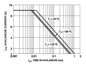
Figure 9. Unclamped Inductive Switching Capability
