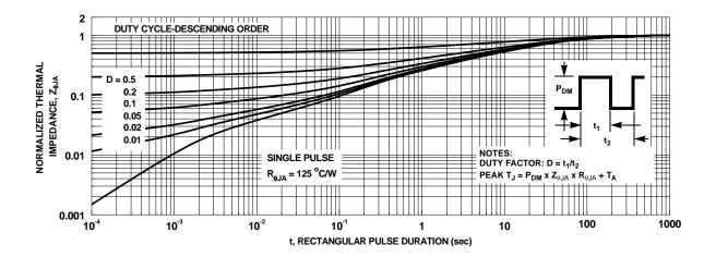
Figure 13. Junction-to-Ambient Transient Thermal Response Curve
