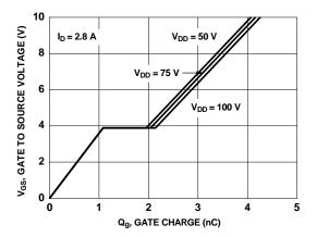
Figure 7. Gate Charge Characteristics
