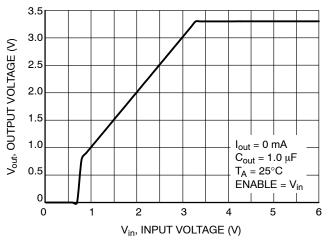
Figure 5. Output Voltage vs. Input Voltage
