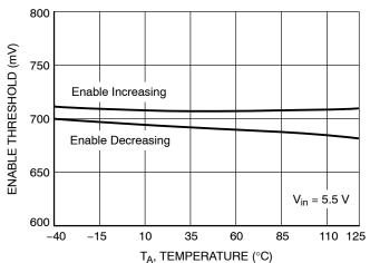
Figure 6. Enable Threshold vs. Temperature
