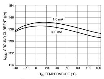
Figure 8. Ground Current vs. Temperature
