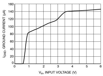
Figure 9. Ground Current vs. Input Voltage
