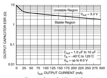
Figure 16. Output Stability with Output Capacitor ESR over Output Current
