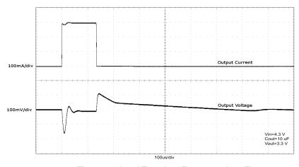
Figure 18. Load Transient Response (10 μF)
