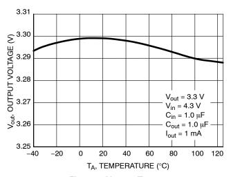
Figure 3. V<sub>out</sub> vs. Temperature
