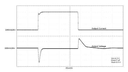
Figure 17. Load Transient Response (1.0  $\mu\text{F}$ )
