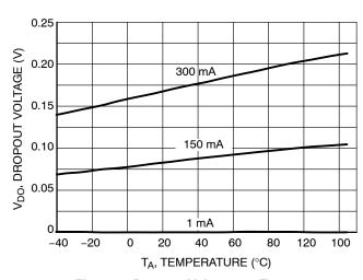
Figure 4. Dropout Voltage vs. Temperature (Over Current Range)
