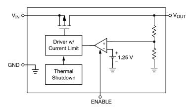
Figure 1. Simplified Block Diagram
