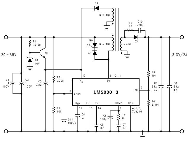
Figure 23. LM5000 Flyback Converter
