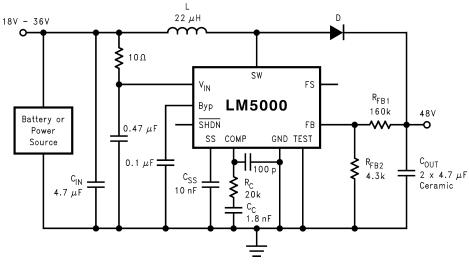
Figure 20. 700 kHz operation, 48V output
