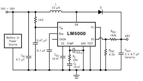
Figure 19. 300 kHz operation, 48V output
