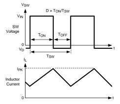
Figure 21. LMR12010 Waveforms of SW Pin Voltage and Inductor Current
