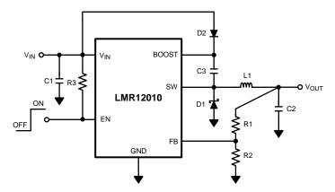
Figure 25. V<sub>BOOST</sub> Derived from V<sub>IN</sub>
