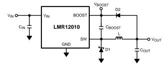
Figure 22. V<sub>OUT</sub> Charges C<sub>BOOST</sub>
