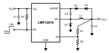
Figure 26. V<sub>BOOST</sub> Derived from Series Zener Diode (V<sub>OUT</sub>)
