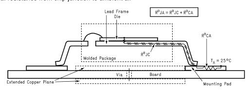
Figure 27. Cross-Sectional View of Integrated Circuit Mounted on a Printed Circuit Board.
