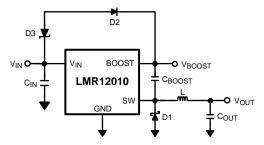
Figure 23. Zener Reduces Boost Voltage from VIN
