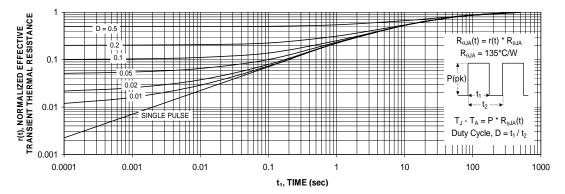
Figure 11. Transient Thermal Response Curve.
