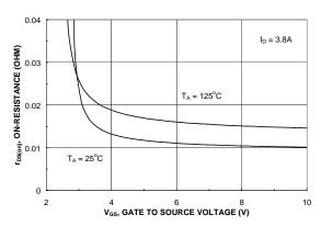
Figure 3. On-Resistance Variation with Temperature.
