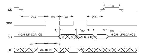
21.4 Waveform 4 – RapidS Mode 3 (F<sub>MAX</sub> = 66MHz)
