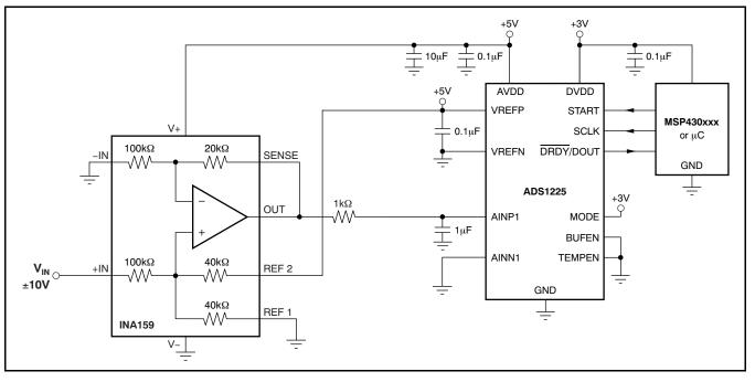
Figure 33. With the Help of an INA159, the ADS1225 Measures ±10V Signals
