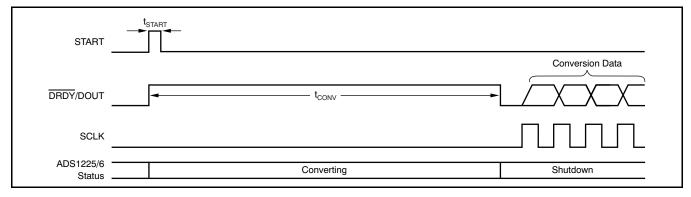
Figure 26. Controlling Conversion with the START Pin
