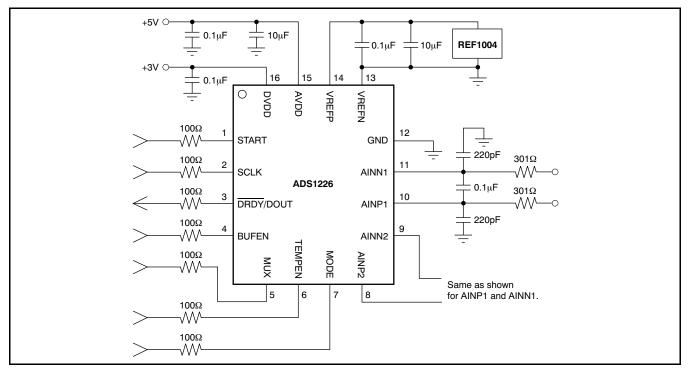
Figure 31. Basic Connections
