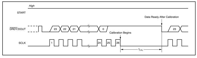
Figure 30. Self-Calibration Timing
