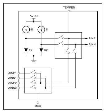
Figure 24. Measurement of the Temperature Sensor in the Input
