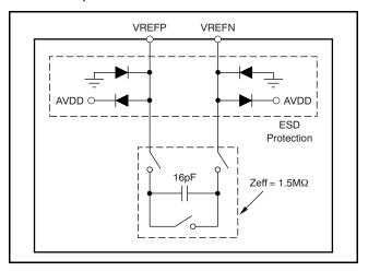
Figure 25. Simplified Reference Input Circuitry
