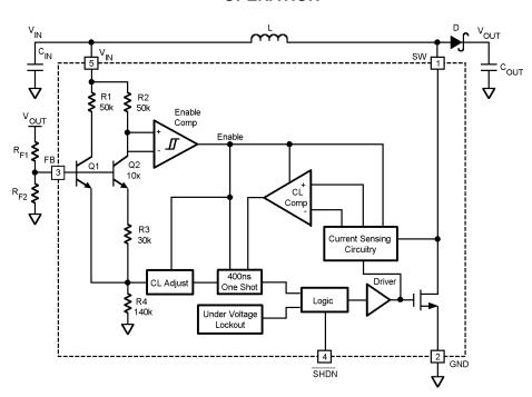
Figure 2. LM2704 Block Diagram
