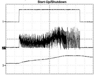
$V_{OUT} = 20V$ ,  $V_{IN} = 2.5V$ 1) SHDN, 1V/div, DC
