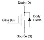
**Remark** Strong electric field, when exposed to this device, can cause destruction of the gate oxide and ultimately degrade the device operation. Steps must be taken to stop generation of static electricity as much as possible, and quickly dissipate it once, when it has occurred.
