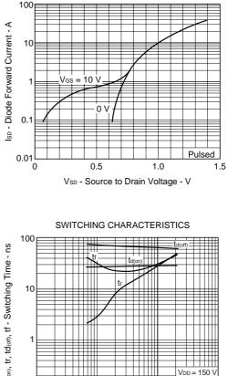
SOURCE TO DRAIN DIODE
