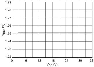
Figure 3.  $V_{REF}$  at  $T_J = 25$ °C
