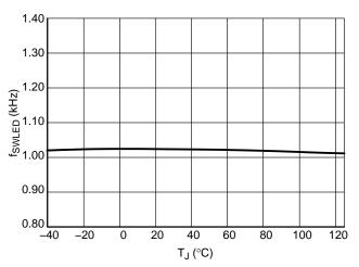
Figure 13. LED Switching Frequency at  $V_{CC} = 15 \text{ V}$
