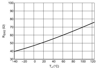
Figure 14.  $R_{SW}$  at  $V_{CC}$  = 15 V
