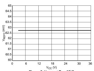
Figure 5.  $V_{REFC}$  at  $T_J = 25^{\circ}C$
