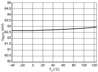
Figure 4.  $V_{REFC}$  at  $V_{CC} = 15 \text{ V}$
