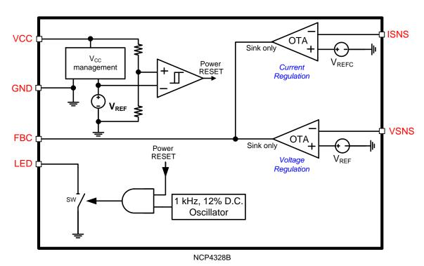
Figure 1. Simplified Block Diagrams NCP4328A and NCP4328B
