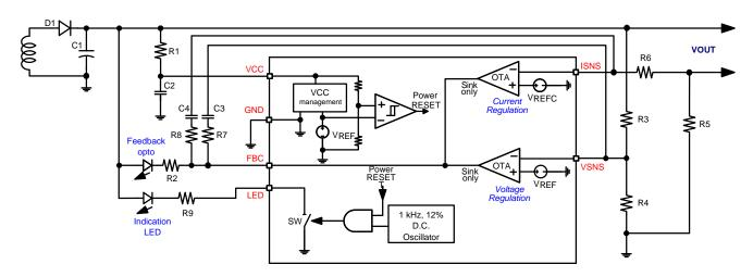
Figure 16. Typical Application Schematic for NCP4328B
