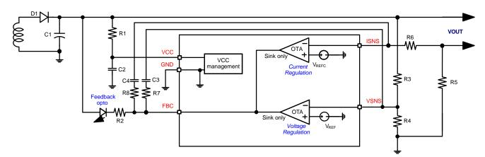
Figure 15. Typical Application Schematic for NCP4328A
