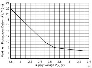
Figure 1. Maximum Propagation Delay vs Supply Voltage
