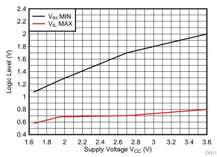
Figure 4. Input High and Input Low Thresholds vs Supply Voltage
