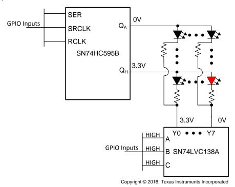
Figure 3. LED Matrix Driver Application
