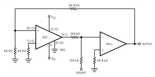
Figure 3. DC Electrical Test Circuit
