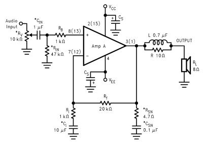
Figure 7. Special Audio Amplifier Application Circuit
