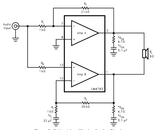
Figure 5. Bridged Amplifier Application Circuit
