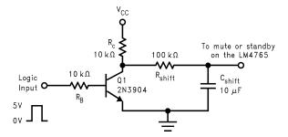
Figure 42. Level Shift Circuit
