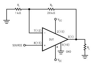
Figure 4. AC Electrical Test Circuit
