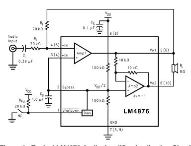
Figure 1. Typical LM4876 Audio Amplifier Application Circuit Numbers in ( ) are specific to the 10-pin VSSOP package.
