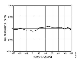
Figure 28. Gain Error Match vs. Temperature
