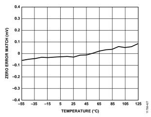
Figure 27. Zero Error Match vs. Temperature
