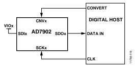
Figure 38. CS Mode, 3-Wire Interface Without a Busy Indicator Connection Diagram (SDIx High)
