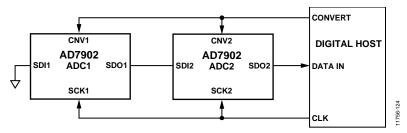
Figure 46. Chain Mode Without a Busy Indicator Connection Diagram
