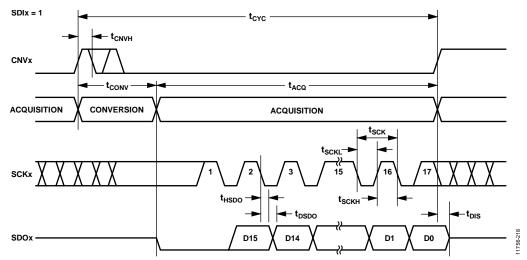
Figure 41. CS Mode, 3-Wire Interface with a Busy Indicator Serial Interface Timing (SDIx High)
