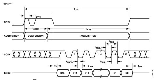
Figure 39. CS Mode, 3-Wire Interface Without a Busy Indicator Serial Interface Timing (SDI High)
