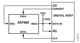
Figure 44. CS Mode, 4-Wire Interface with a Busy Indicator Connection Diagram
