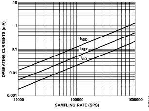
Figure 37. Operating Currents per ADC vs. Sampling Rate
