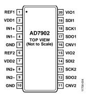
Figure 4. Pin Configuration
