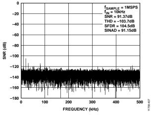
Figure 7. FFT Plot,  $V_{REF} = 5 V$
