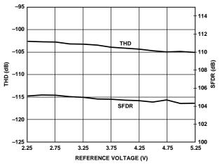
Figure 16. THD and SFDR vs. Reference Voltage
