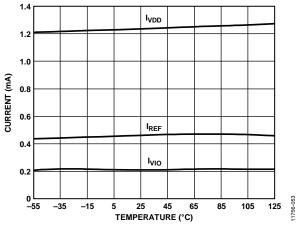
Figure 23. Operating Currents for Each ADC vs. Temperature
