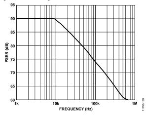
Figure 36. PSRR vs. Frequency
