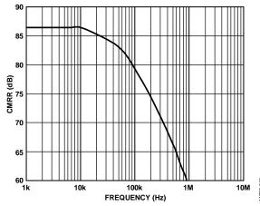
Figure 34. Analog Input CMRR vs. Frequency
