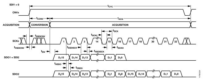
Figure 47. Chain Mode Without a Busy Indicator Serial Interface Timing
