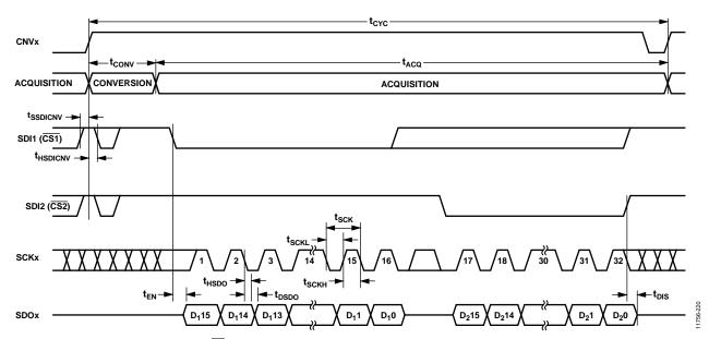
Figure 43. CS Mode, 4-Wire Interface Without a Busy Indicator Serial Interface Timing
