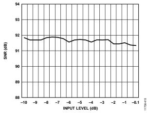
Figure 15. SNR vs. Input Level
