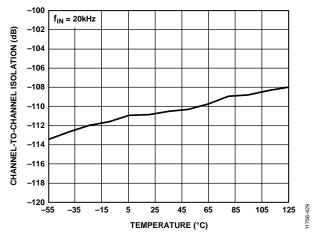
Figure 29. Channel-to-Channel Isolation vs. Temperature
