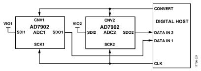
Figure 50. Potential Simultaneous Sampling Connection Diagram
