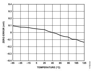
Figure 24. Zero Error vs. Temperature
