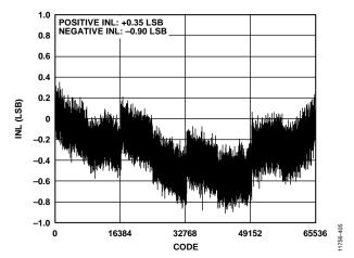
Figure 5. Integral Nonlinearity vs. Code,  $V_{REF} = 5 V$
