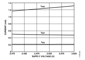
Figure 19. Operating Currents for Each ADC vs. Supply Voltage
