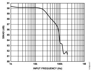
Figure 17. SINAD vs. Input Frequency
