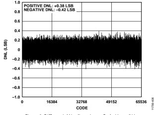
Figure 8. Differential Nonlinearity vs. Code,  $V_{REF} = 5 V$
