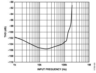
Figure 20. THD vs. Input Frequency
