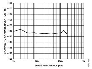
Figure 30. Channel-to-Channel Isolation vs. Input Frequency
