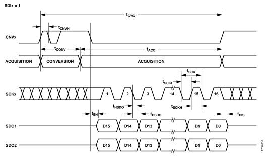
Figure 51. Potential Simultaneous Sampling Serial Interface Timing
