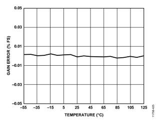
Figure 25. Gain Error vs. Temperature
