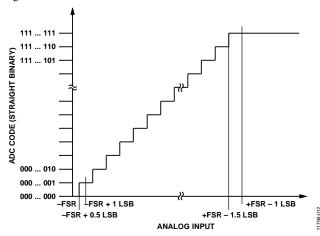
Figure 32. ADC Ideal Transfer Function
