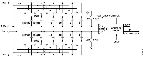
Figure 31. ADC Simplified Schematic
