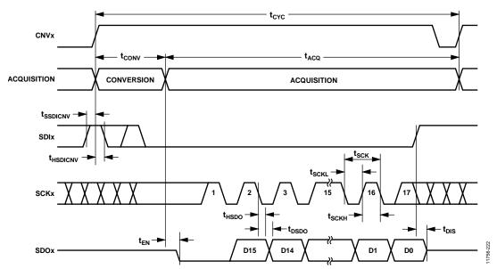
Figure 45. CS Mode, 4-Wire Interface with a Busy Indicator Serial Interface Timing
