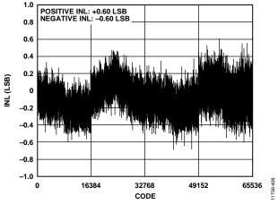
Figure 6. Integral Nonlinearity vs. Code,  $V_{REF} = 2.5 V$
