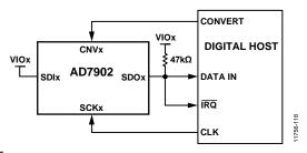
Figure 40. CS Mode, 3-Wire Interface with a Busy Indicator Connection Diagram (SDIx High)
