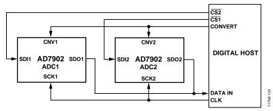
Figure 42. CS Mode, 4-Wire Interface Without a Busy Indicator Connection Diagram
