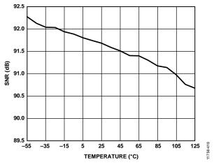
Figure 18. SNR vs. Temperature
