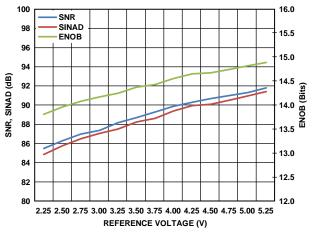
Figure 13. SNR, SINAD, and ENOB vs. Reference Voltage
