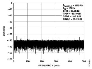
Figure 10. FFT Plot,  $V_{REF} = 2.5 V$
