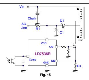
A 230nS leading-edge blanking (LEB) time is included in the input of CS pin to prevent the false-trigger from the current spike. In the low power applications, if the total pulse width of the turn-on spikes is less than 230nS and the negative spike on the CS pin below -0.3V, the R-C filter is free to eliminate. (As shown in Fig.16).
