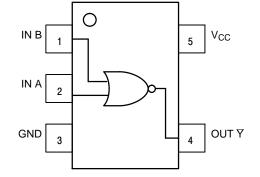
Figure 1. Pinout (Top View)
