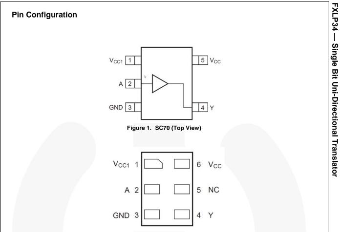
Figure 2. MicroPak<sup>™</sup> (Top Through View)
