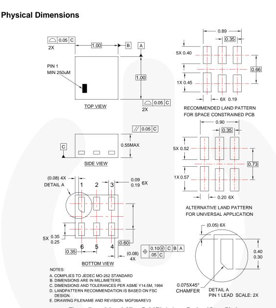
Figure 7. 6-Lead, MicroPak2™, 1x1mm Body, .35mm Pitch
