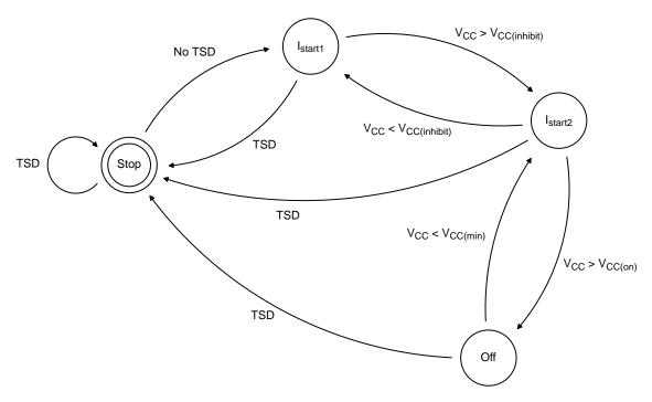
Figure 48. HV Start-up Current Source State Diagram
