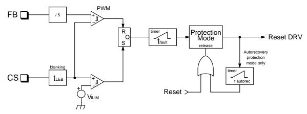
Figure 40. Timer-Based Overcurrent Protection
