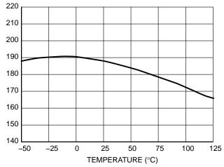
Figure 26. Current I<sub>NTC(SSTART)</sub> Sourced from the Latch Pin, During Soft-Start
