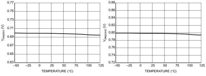
Figure 15. FB Pin Skip-in Level V<sub>skip(in)</sub>
