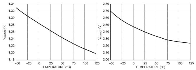
Figure 23. Latch Pin Open Voltage V<sub>clamp0</sub>
