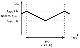
Figure 30. Frequency Jittering
