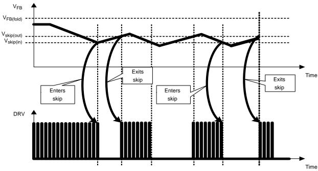
Figure 45. Skip Cycle Timing Diagram
