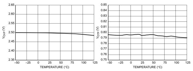
Figure 21. Latch Pin High Threshold VOVP
