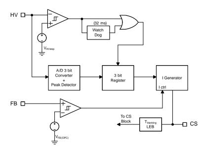
Figure 35. Schematic Overpower Compensation Circuit
