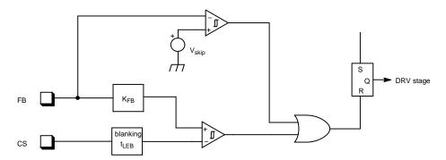
Figure 44. Skip Cycle Schematic
