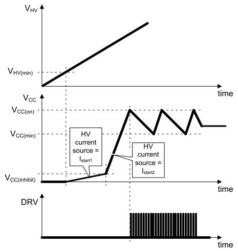
Figure 28. Start-up Timing Diagram
