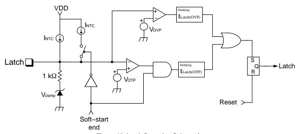
Figure 46. Latch Detection Schematic
