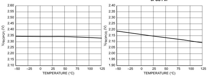
Figure 19. FB Pin Level V<sub>FB(OPCF)</sub> Above Which is the Overpower Compensation Applied
