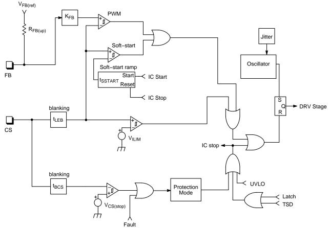
Figure 32. Current Sense Block Schematic
