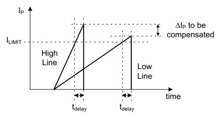
Figure 34. Line Compensation for True Overpower Protection
