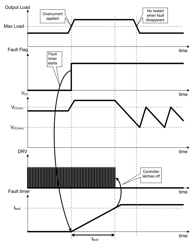
Figure 42. Latched Timer-Based Overcurrent Protection
