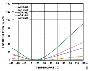
Figure 11. Line Regulation vs. Temperature
