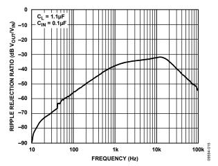
Figure 15. ADR3525 Ripple Rejection Ratio vs. Frequency
