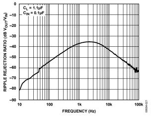
Figure 21. ADR3550 Ripple Rejection Ratio vs. Frequency
