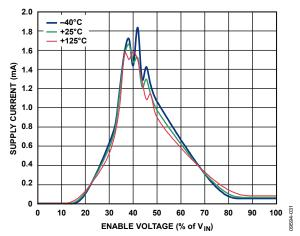
Figure 31. Supply Current vs. ENABLE Pin Voltage
