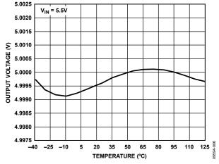
Figure 6. ADR3550 Output Voltage vs. Temperature
