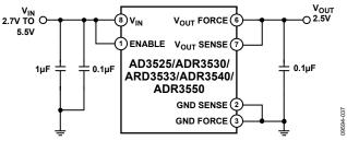
Figure 37. Basic Reference Connection
