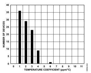
Figure 4. ADR3525 Temperature Coefficient Distribution
