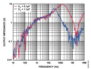
Figure 32. ADR3550 Output Impedance vs. Frequency
