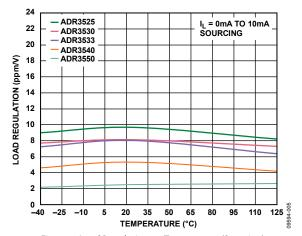
Figure 5. Load Regulation vs. Temperature (Sourcing)
