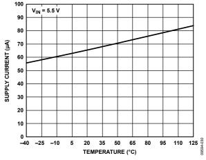
Figure 30. Supply Current vs. Temperature
