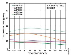
Figure 8. Load Regulation vs. Temperature (Sinking)
