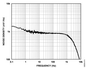
Figure 14. ADR3525 Output Noise Spectral Density
