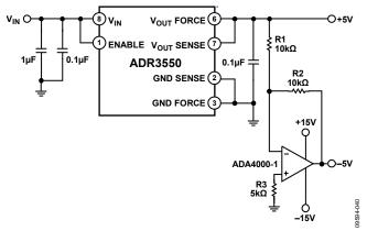
Figure 40. ADR3550 Bipolar Output Reference
