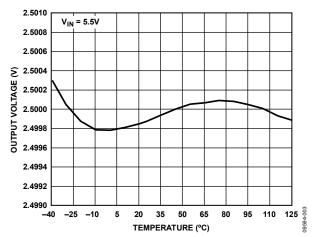
Figure 3. ADR3525 Output Voltage vs. Temperature
