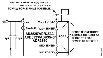
Figure 38. Application Showing Kelvin Connection
