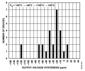
Figure 34. ADR3550 Thermally Induced Output Voltage Hysteresis Distribution
