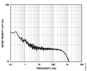
Figure 20. ADR3550 Output Noise Spectral Density
