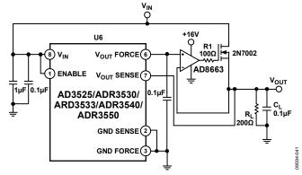
Figure 41. Boosted Output Current Reference
