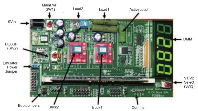
Figure 1. Hardware Components
