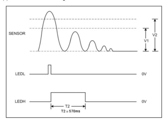
[Note]: (1) There interval of output pulse (LEDL or LEDH) between different trigger must large then 50ms.
