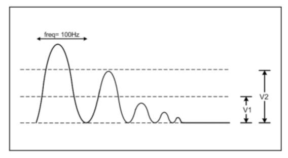
The trigger point of first sensational range is V1 1.6mV, and the frequency is 100Hz. This trigger point was be designed in chip, you must adjust the strength of sensor circuit to fit the trigger point.
