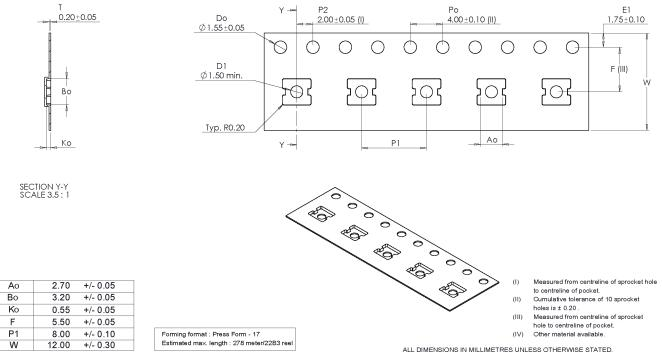
(1) Pin 1 is oriented in the top-left quadrant of the tape enclosure (closest to the carrier tape sprocket holes).
