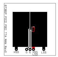
Max  $R_{\theta JA} = 84^{\circ}C/W$ when mounted on 1 inch<sup>2</sup> (6.45 cm<sup>2</sup>) of 2 oz. (0.071 mm thick) Cu.
