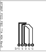
Max  $R_{\theta JA} = 184^{\circ}C/W$ when mounted on minimum pad area of 2 oz. (0.071 mm thick) Cu.
