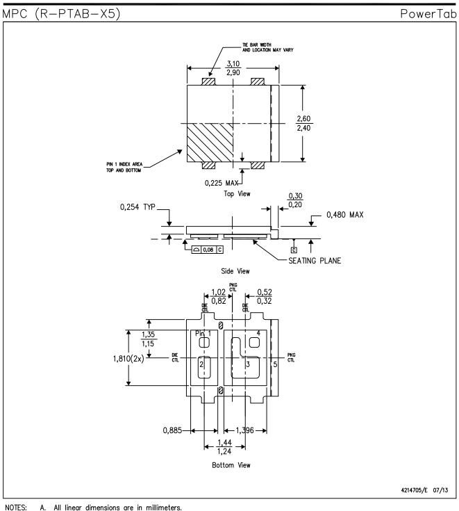
A. All linear dimensions are in millimeters.
