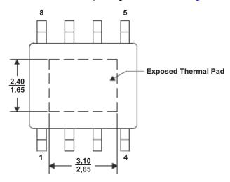
Figure 22. Thermal Pad Dimensions
