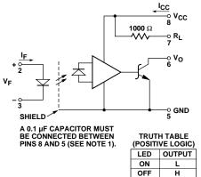
A 0.1 pF bypass capacitor must be connected between pins 5 and 8.
