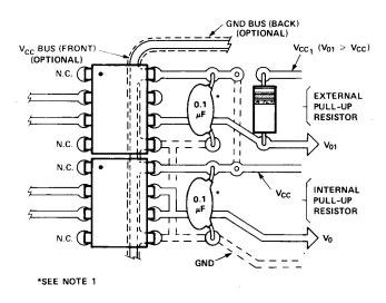
Figure 19. Recommended Printed Circuit Board Layout.
