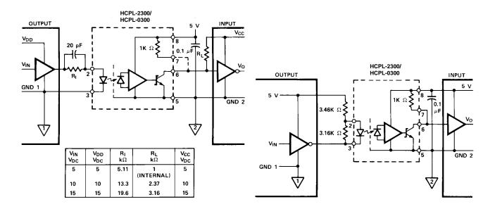
Figure 13. Active CMOS Series Drive Circuit.
