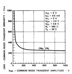
Figure 9. Typical Common Mode Transient Immunity vs. Common Mode Transient Amplitude.
