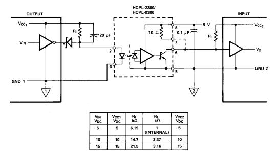
\*SCHOTTKY DIODE (HP 5082-2800, OR EQUIVALENT) AND 20 pF CAPACITOR ARE NOT REQUIRED FOR UNITS WITH OPEN COLLECTOR OUTPUT.
