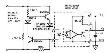
Figure 18. RS-232-C Interface Circuit with HCPL-2300/ HCPL-0300. 0°C <  $T_A$  <  $85\,^{\circ}C.$
