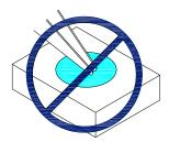
3. Do not stack together assembled PCBs containing exposed LEDs. Impact may scratch the silicone lens or damage the internal circuitry.
