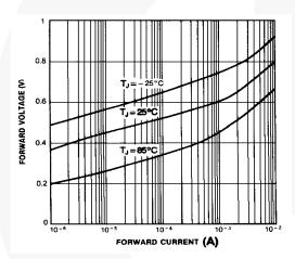
Figure 5. Forward Characteristics
