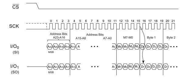
Figure 7-5. Dual-I/O Read Array (Previous command set M5, M4 = 1,0)
