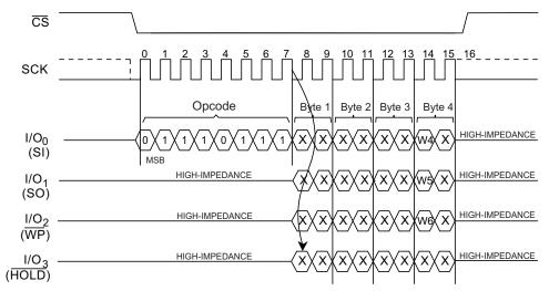
The Set Burst with Wrap instruction sequence is:  $\overline{CS}$  goes low  $\rightarrow$  Send Set Burst with Wrap instruction  $\rightarrow$  Send 24 Dummy bits  $\rightarrow$  Send 8 "Wrap bits"  $\rightarrow$   $\overline{CS}$  goes high.
