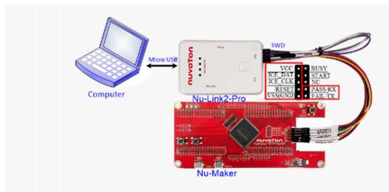
(2) Find the Nu-Link2 Virtual Com Port at Device Manger. Nu-Link2-Pro can directly use the virtual serial port (VCOM) function without any settings.
