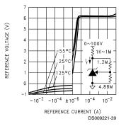
Reference Voltage vs Current and Temperature
