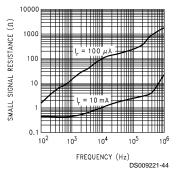
Typical Performance Characteristics (Reference) T<sub>J</sub> = 25°C, FEEDBACK pin shorted to V<sup>-</sup>
