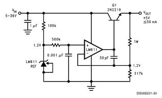
FIGURE 13. Simple Low Quiescent Drain Voltage Regulator. Total Supply Current is approximately 320  $\mu$ A when V<sub>IN</sub> = 5V, and output has no load.
