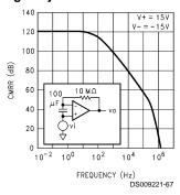
**Negative Power Supply** Voltage Rejection Ratio
