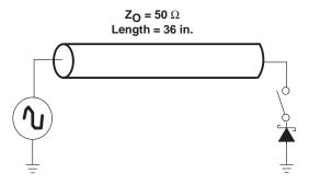
Figure 5. Diode Test Setup
