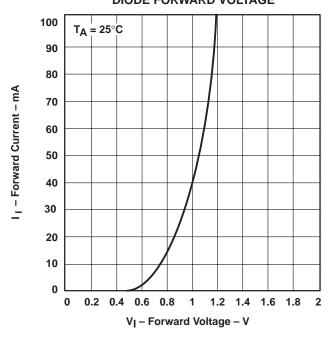
Figure 4. Typical Input Current vs Input Voltage (Upper Diode)
