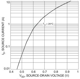
Fig. 8 Diode Forward Voltage vs. Current
