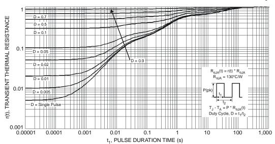
Fig. 11 Transient Thermal Response
