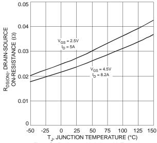
Fig. 6 On-Resistance Variation with Temperature
